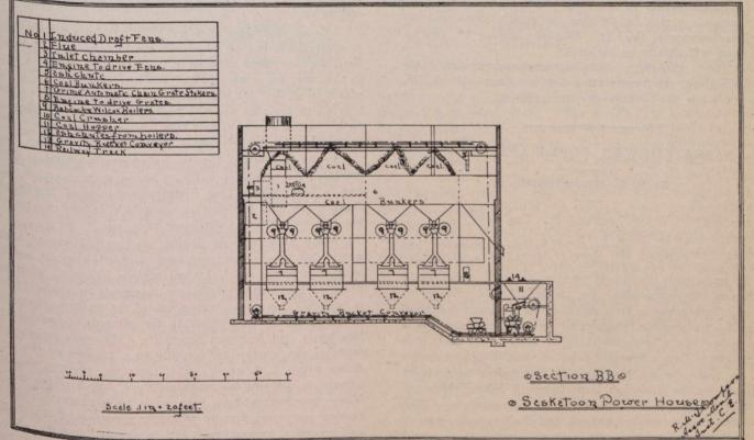
extend down to the hoppers of the stokers, and a steady flow of coal for the hoppers of the stokers at all times. The of coal from above supplies the stokers at all times. The overhead bunkers are kept filled by a gravity bucket con-
