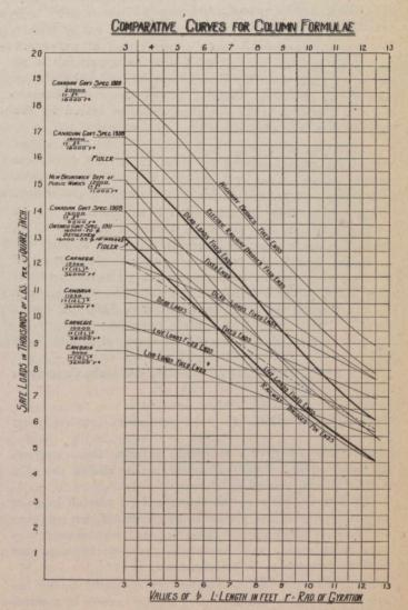
The other two curves belonging to the same specification -one for electric railway bridges and the other for railway bridges-would be reduced in a similar manner, but have not been shown.
