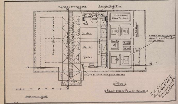
buildings of this class, and is eminently fitted for the economical and convenient handling of the work. It is designed to admit of the extension of the plant up to 4,000 tion with the economizers, will deliver 650 b.h.p. to the engines, or a total of 2,000 horse-power. These boilers are equipped with Grime automatic chain grate stokers, which are driven by an independent engine, and feeds the coal as required under the boilers to convey the coal to the stokers.
