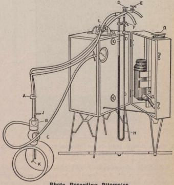
Photo Recording Pitometer.
