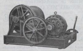
The Electric Hoist in this illustration has the drum keyed fast to the shaft. It cannot turn in any direction except it is driven by the motor. There is no possibility of accidents through worn or loose frictions. The Hoist is under absolute control of the operator at all times.
