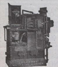
and it will instantly show any improvement in evaporation due to better fuel, better methods of firing, better condition of heating surfaces (removal of soot and scale), better condition of boiler setting (stopping up air leaks), etc.
