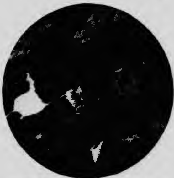
Photomicrograph showing eutaxitic structure in a basalt flow occurring on the portage from Dufresnoy to Sills lake. Ordinary light. Magnified 20 diameters.
