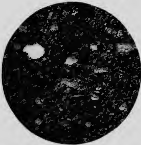
Photomicrograph of the greywacke of the Pontiac series, occurring on Clericy lake, Pontiac county, Que. Crossed nicols. Magnified 20 diameters. Compare with Plates XVII and XVIII.
