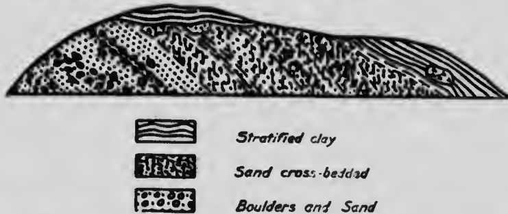
Fig. 6. Diagrammatic section through kame on the National Transcontinental railway in range VII, La Sarre township.
