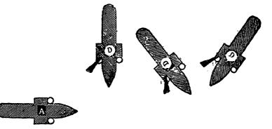
If A sees a White Mast-head Light above the Green Light, A knows that the vessel is a steam-vessel, and is either approaching her in the same direction as B, or is crossing to starboard in some direction, as D D D. 22 V. (1859) c. 19. Schedule.
