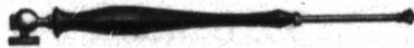
No. 9.—The same, shown with brush pushed within its cylinder for protection when not in use.
