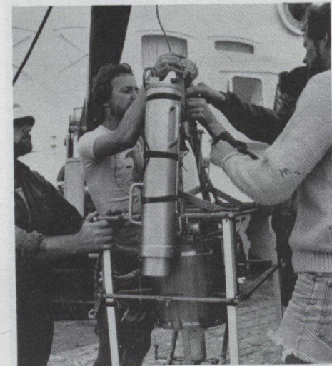
Scientists and crew of the Hudson are preparing the Patterson-Schaule sampler used for the collection of uncontaminated sea water to measure the amount of trace metals.
