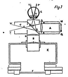
A tube C of the same width, 1½ inches in length, is joined to the side of the outer extremity of the tube B opposite to and in a line with tube A. The outer extremity of the tube B extends ¼ of an inch beyond its juncture with the tubes A and C, and is terminated by a thin brass diaphragm having a central circular aperture of ¾ of an inch in diameter.
