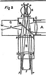
Reflection. — Let E (fig. 2) represent the same eye illuminated as just described, D the plate glass, and H I the lenses in the camera tube. Rays from any portion of the illuminated fundus as a, are reflected from the fundus and emerge from the cornea at b c, the width of the dilated pupil, and proceed to the plate glass D (parrallel rays of lightemerging from an eye having its accommodation paralyzed are parral-
