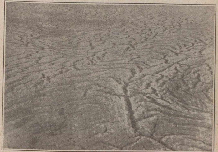
FIG. 6—SLUDGE AFTER IT HAS BEEN IN THE DRYING BED FOR THIRTEEN DAYS
