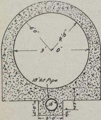
Fig. 2.—Concrete Section in Open Cut.
