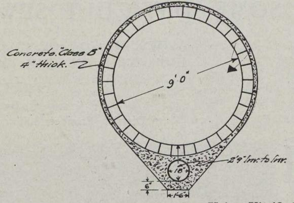
Fig. 4.—Alternative Section, Using Vitrified Segment Sewer Blocks.
