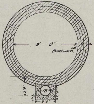
Fig. 3.—Brick Section in Tunnel.
