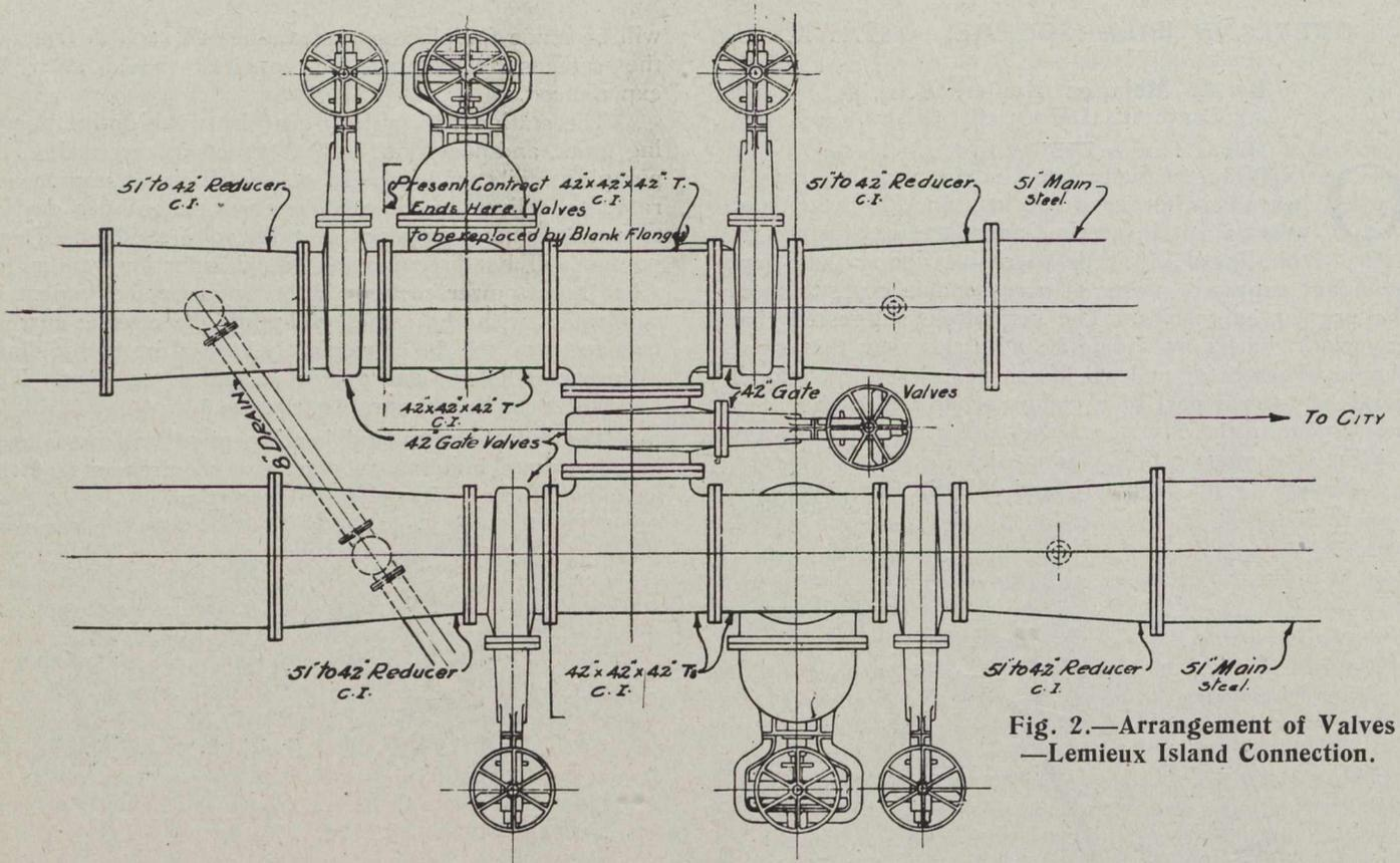
Fig. 2.—Arrangement of Valves—Lemieux Island Connection.
