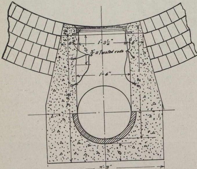
Fig. 8.—Type of Manhole on the 18-inch Vitrified Pipe Sewer.
