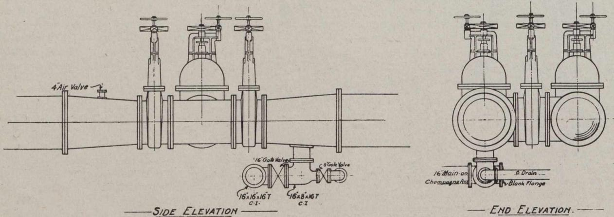
Fig. 3.—Wellington Street Junction of the Two 51-inch Pipes with the Single 51-inch Pipe Line.
