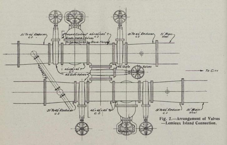
settled, the pipes can then be connected without interferring in any way with the city's supply. It is to be noted that 51-inch x 42-inch reducers were placed at each valve. This procedure effects a considerable reduction in cost and is considered to be quite as satisfactory. By shutting off the alternate set of valves, repairs or tests can be made
