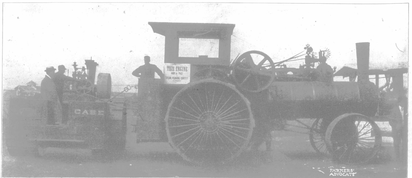
GOLD MEDAL WINNER, CLASS D, FOR STEAM ENGINES AT WINNIPEG INDUSTRIAL EXHIBITION, PLOWED 3.62 ACRES IN 1 HR. AND 50 SECONDS, USING 442 LBS OF COAL AND 361 GALLONS OF WATER. THE SMALL ENGINE WON GOLD MEDAL IN CLASS FOR 20 HP. TRACTION ENGINE AT BRANDON EXHIBITION.
