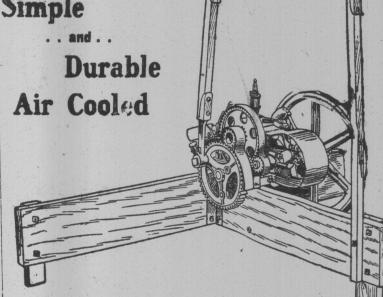
It has no water jacket. Designed to take the place of the man at the pump. Any one who watches this outfit pump water for 15 minutes will never again be will ing to work the pump handle. Will connect with any style of pump which is already in the well. Supplied for setting up complete. A simple, durable pumping engine at low cost. Sold by
