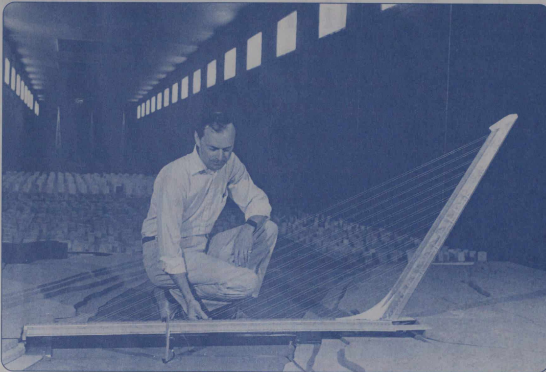
Peter King, engineering professor at the University of Western Ontario, surveys scale model of the Alamillo bridge in wind tunnel environment.
