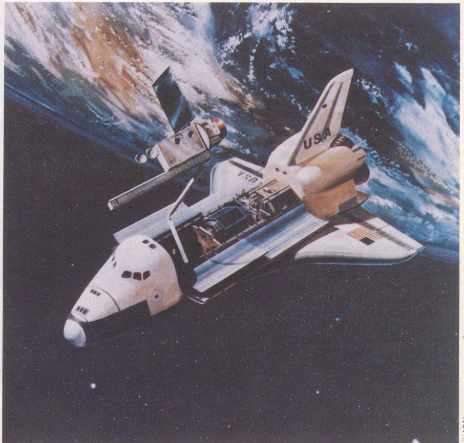
At work, Canadarm will retrieve satellites or place them in orbit. The arm can also be used to inspect the Shuttle while in orbit.
