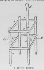
are 12 inches long and notched at the top so the bar on which the spool is hung can rest as shown. Lever d regutates the speed of turning or paying out ...ire by pressing against the roll. The whole outfit is set in the ground at an end of the proposed fence, spool put in place and a horse with singletree attached to end of wire. The horse can be ridden or led by a man, while a boy operates the lever.—R. G. Melson, in Farm and Home.
