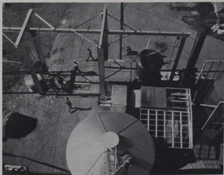
Left, waste wood is converted to flammable gas in Saskatchewan Forest Products' fluid bed gasifier at Hudson Bay. Bottom left, natural fermentation will create methane in this 23,000-gallon anaerobic digester. Below, large straw bales are burned to dry grain and heat buildings.
