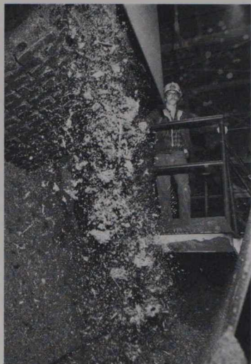
Several lumber companies in British Columbia burn hog fuel to power their mills. Bark, sawdust and waste wood are hogged (chopped up), and moisture is pressed out. Left, the prepared hog fuel comes out of the press at the MacMillan Bloedel mills at Port Alberni. Right, hog fuel is piled outside the British Columbia Forest Products mill at Crofton on Vancouver Island.
