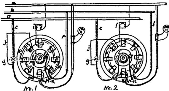
a Positive bus bar. b. Equalizing bar. c Negative bar. d. Commutators. e. Armatures. f. Brushes. g. Circuit breaker. h. Ammeter. i. Rheostat. j. Shunt field. k. Series field. r. German silver resistance.
