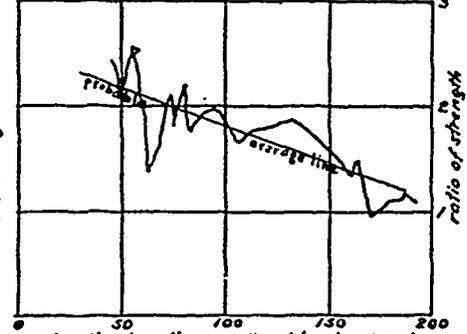
Diagram 5. Ratio of Rammed to Pressed 3 to 1 Sand Tests.
