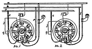
a Positive bus b.r. b. Equalizing bar. c Negative bar. d. Commutators. c. Armatures. f. Brushes. g. Circuit breaker. h Ammeter. i. Rheostat. j. Shunt field. k. Seric. field. r. German silver resistance.
