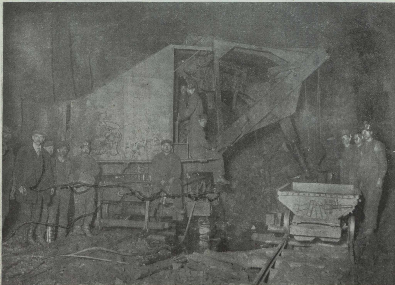
The Electric Shovel, Loading Iron-ore into Mine-car in the Scotia No. 3 Mine at Wabana, Newfoundland.
