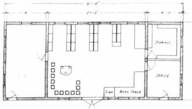
PLAN OF CENTRAL RESCUE STATION, SHOWING APPARATUS
