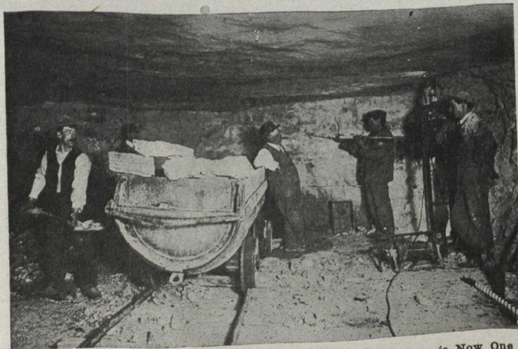
"Alabastine," Made from Clay, Sand, Lime, Hair and Gypsum, is Now One of the "Household Words." This is a View of a Gypsum Mine at Caledonia, Near Hamilton. Operated by the Alabastine Company of Paris.
