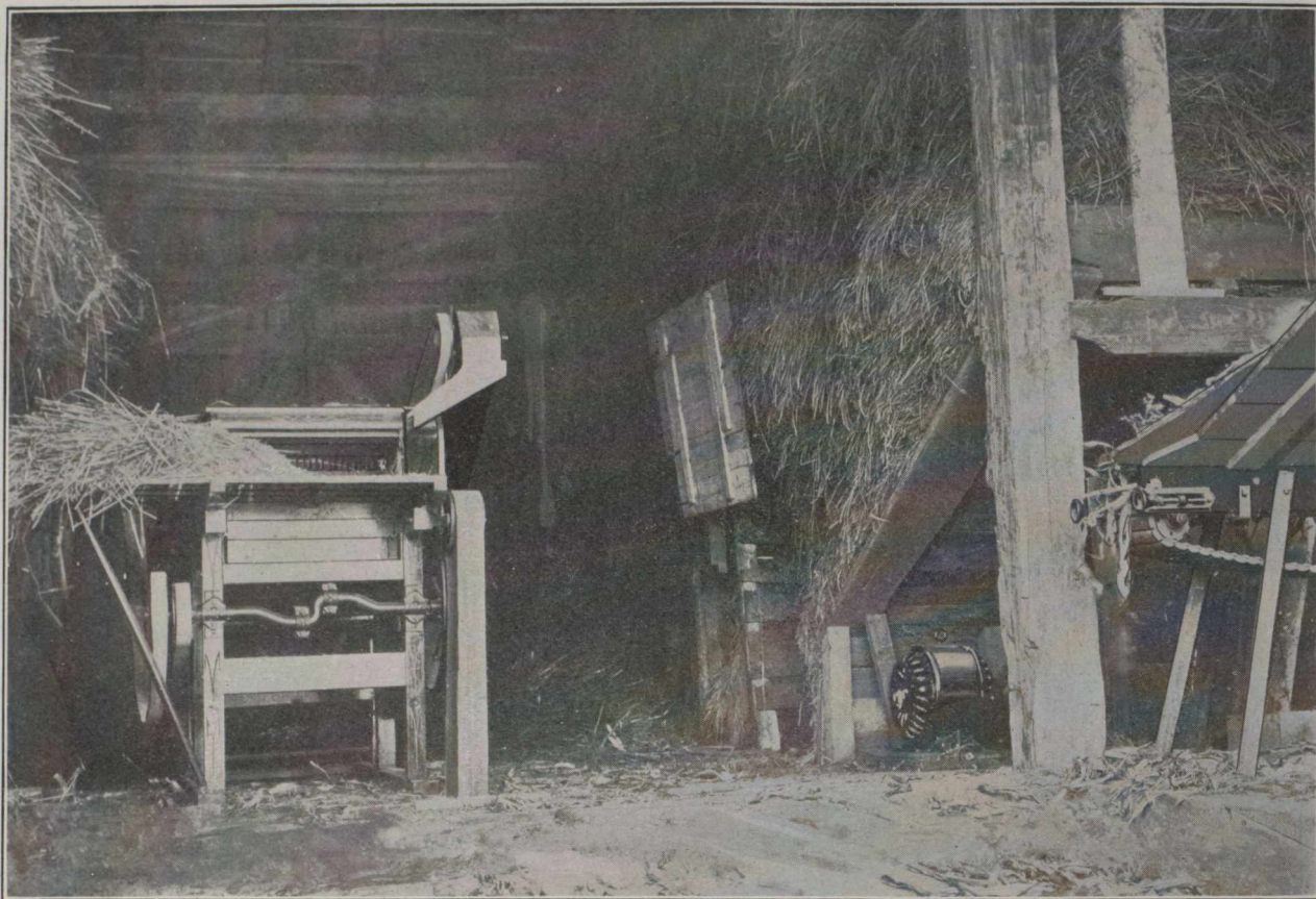
Separator and cutting box driven by 5 H. P. motor at Mr. Clark's farm.
