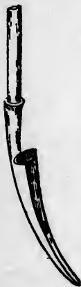
FIGURE 16. Finishing Scoop for shaping bottom of drain ditch to proper grade and of correct form to receive tile.
