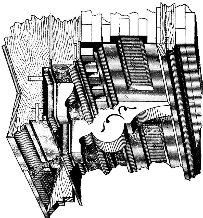
FIG. 1.—APPROVED CONSTRUCTION, USING WOOD LOOKOUTS.
