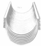
Pedlar Culverts are shipped in half-sections, nested—saving freight and making carriage easy in roughest country. Quickly and easily transported anywhere. Fig. 1 shows the half-sections or semicylinders, nested one within the other for shipment. One of the ribs is a radial flange, the other a re-curved flange. Sections are assembled as shown by Fig. 2. Note that the ribs are flat, and the
