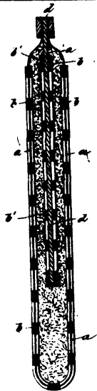
18256 Fitzgerald's Secondary Battery of Accumulator.
