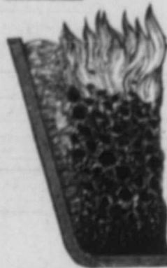
Usual sloping wall firepot. Blanket of ashes absorbing heat.
