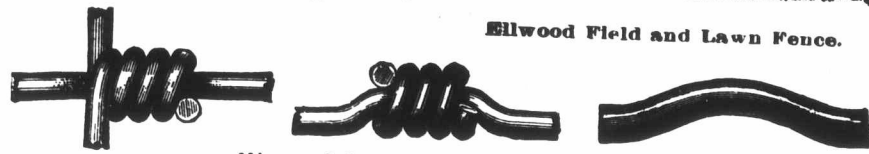
Large Joints and Tension Curves.
