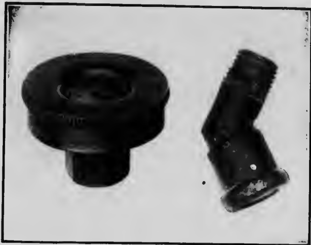
Fig. 27.—A good type of nozzle and an elbow to control the direction of the spray.
