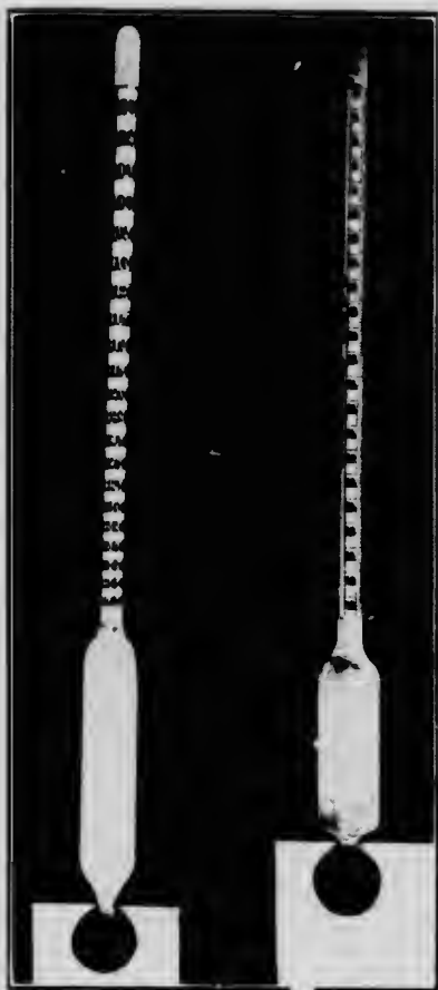
Fig. 8. Hydrometers (about \frac{1}{2} g. e). The one on the left has specific gravity, the other Baumé, readings.
