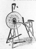
Grindstone. It runs like a bicycle You sit down on the seat and wor the treadles with both feet. ing of tools of all kinds. It also en ter work: has self-watering attachmen eat adjustable in height stone can be adjusted on frame.
