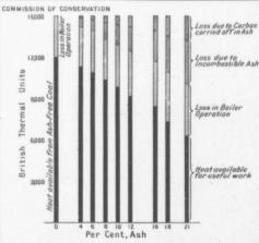
REDUCTION IN HEAT VALUES DUE TO PRESENCE OF ASH IN COAL
