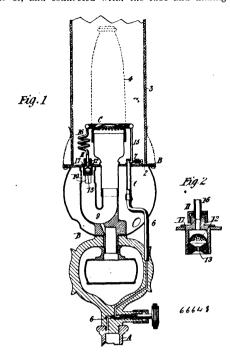
6th. A vapour jet fitting consisting of a perforate non-metallic mineral, substantially as described. 7th. A vapour jet fitting consisting of a piece of quartz or crystal with a polished orifice therethrough.
