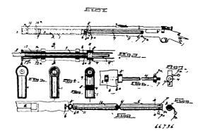
with a sliding bayonet, an operating rod removably attached to the handle of said bayonet, a sheath surrounding said rod, a lever for rotating the rod, a cam fixed to said rod and adapted to rotate by the movement of said lever, and a bayonet sheath having recesses adapted to engage the projecting portion of said cam and to lock the bayonet in position, substantially as described.
