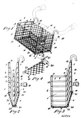
having extensions from same terminating in hooks, and an adjustable tastening device to encircle the head post of the bicycle, said adjustable fastening device being itself adjustable in its connection to the rear end of the carrier.
