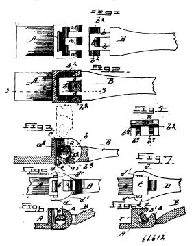
a shaft portion having shanks bb, cross head  $b^1$ , lugs  $b^2b^2$ , and shoulder  $b^3$ , substantially as and for the purpose described.
