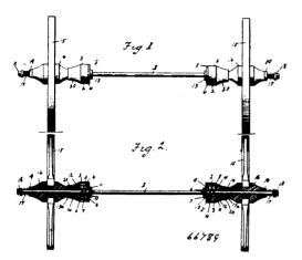
upon the extremity of the axle, a compression plate imposed against the outer end of the hub, and a spring intermediate of the compression plate and nut, substantially as specified.
