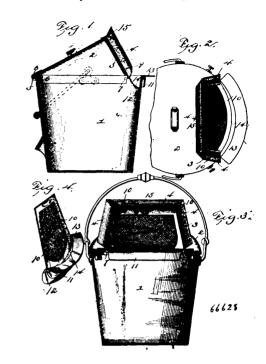
catches for securing the cover to the pail and the strainer plate to the cover, substantially as described.
