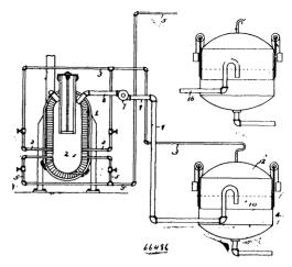
gases from the smelting furnace 1 and return pipes 3 and 5 connecting said gasometers and said smelting furnaces.
