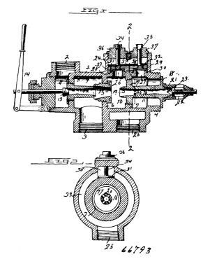
tube secured to the partition between the suction and cold water overflow chambers, of a condensing or delivery tube having lateral perforations therein, a flange thereon secured to the partition between the cold and hot water overflow chambers, a disc thereon abutting against the rear end of said shell, closing the rear end of said hot water overflow chamber, and a deck valve in said condensing or delivery tube.
