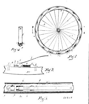
end rigidly connected to the inner rim b, a spiral spring k, made to surround the wires g, and impinge on the slide plates h, and the rear block e, substantially as specified.
