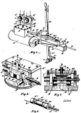
frame as and for the purpose specified. 5th The combination with the cylinder provided with inlet ports, the steam chest and the adjustable portion of the valves, of the block M¹ provided with serpentine grooves m, the block O fitting in a recess in the block M, the block F fitting in the block O and the set screw extending through the valve chest into the recess in the block P, as and for the purpose specified.
