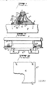
shoulder of the rail at the top, in combination, substantially as shown and described.
