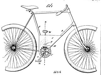
terminating between said second and third gear wheels and provided with a handle within the plane of the frame of the bicycle whereby said second and third gear wheels may be moved into and out of engagement with said first and fourth gear wheel, substantially as shown and described.
