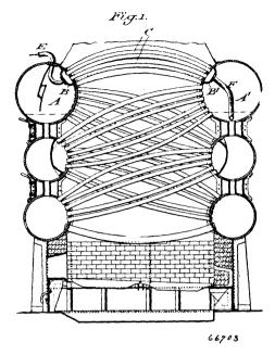
tioned side tubes, hollow casings located within the top drums for receiving the ends of the feed water heating tubes, a feed water inlet pipe leading to one of the hollow casings and a feed water outlet pipe leading from the other of the hollow casings and in open communication with the interior of the drum within which it is located, substantially as set forth.
