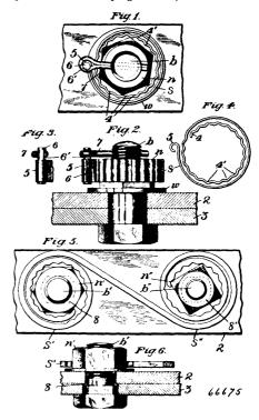
ing locking spring seated at its free end in the recess in the bolt and having in its inner face a recess for receiving a corner of the nut.
