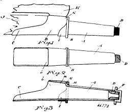
projecting from the underside of the sheath to underlap the axle tree, an abutting collar fitted on the axle arm and bearing against the shoulder, a flange projecting from the collar underlapping the adjacent end of the sheath, and a plug fitted into the end of the axle arm to receive the axle nut, substantially as specified.
