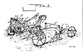
passing transversely through said bar, a frame supported by said threaded rod, the lower end of said rod forming the axle, substantially as described. 4th. A gang plough comprising a frame, a draft plate secured thereto having a plurality of perforations, a draft plate secured to said bar by means of a pin passing therethrough and engaging one of said perforations, a clevis pivoted to said draft plate, and a ter rod connecting said plate with the frame, substantially as described.
