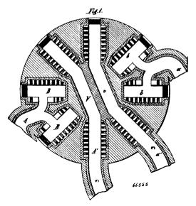
neath the hearth and round the common centre of the furnace, all as a means of obtaining the maximum working space for the attendants and the maximum utilization of the heating fuel.
