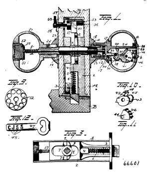
cut out portion to form shoulders, and a lug or projection on the button adapted to be held against either one of said shoulders to hold the rod in or out of engagement with the outer knob.
