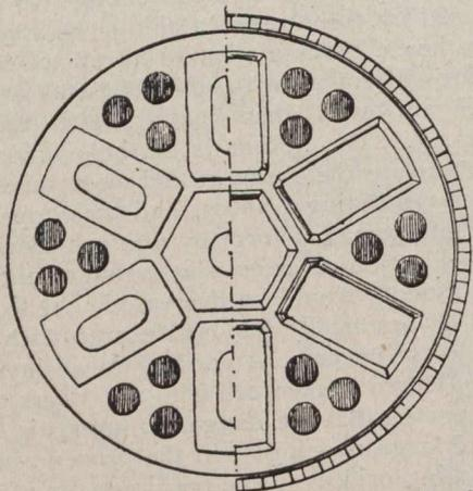
Fig. 4.—Manhole Cover With Circular Perforators (by Falkenroth).
