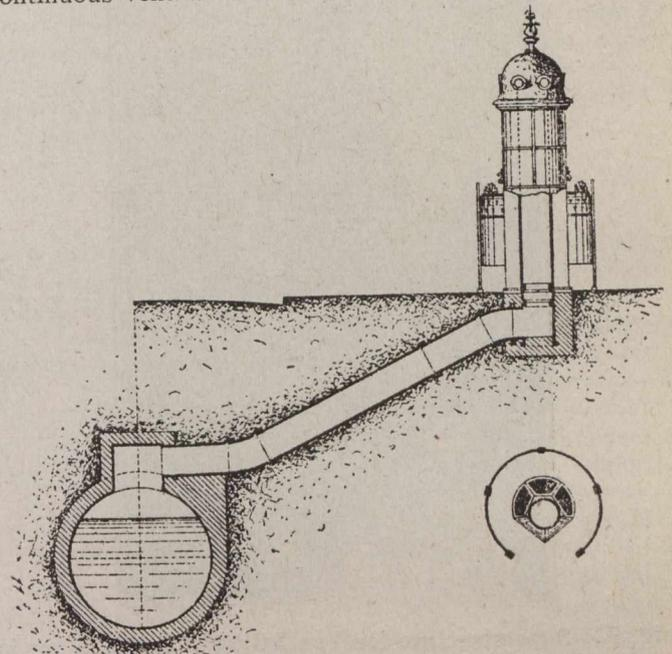
Fig. 6.—Ventilating Device on a Paris Trunk Sewer.
