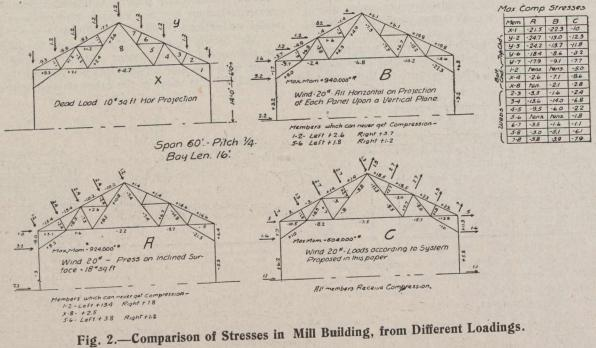
is equal to the product of the area of the surface by the square of velocity, multiplied by the co-efficient 0.14.
