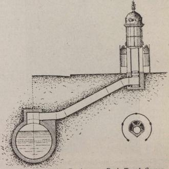
Fig. 6.—Ventilating Device on a Paris Trunk Sewer.
