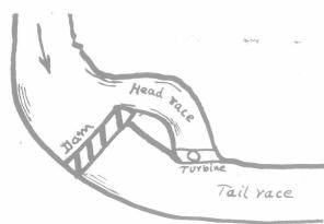
A Dam for Turbine Installation.
