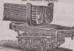
60—Bogie Wagon, with Swivel Fork for carrying Long Balke
