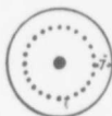
Dots indicate Oak Plugs. From plugs to front of wheel about 7" to 8"
