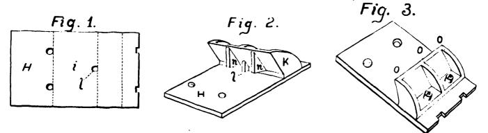
Figure 1 is a seat view of the Chair, showing the place of the rail, the place of the chair back, and places for the spikes. Figure 2 is the seat and back of the Chair, showing the front side of the back, with riles for keeping the rails from displacement. Figure 3 is the Chair (position changed), showing the heads of the rivets uniting the seat and back, and the ribs that strengthen the back and protect the Chair.
