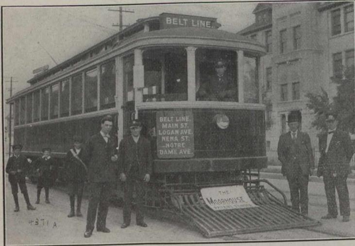
The Moorhouse Car Fender, tripped (fully covered by patents)
