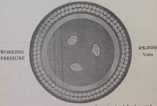
No. 1/0 B. & S. Gauge, Three Conductor, Paper-insulated, Lead-covered, Double-wire Armoured, Sub-marine Cable built to the Specification of R. S. Kelsch, Esq., Consulting Engineer, Montreal.
