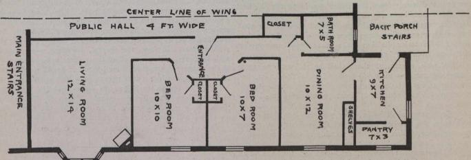
Sketch showing typical floor plan of five-room suite with Public Hallway, one suite on each side of hall. No fire wall dividing the wing of the building.
