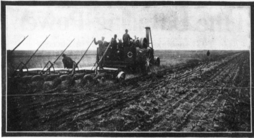
The Sawyer-Massey 32 h.p. Steam Tractor pulling 10 John Deere Plows (Silver Medal winner Class B)
