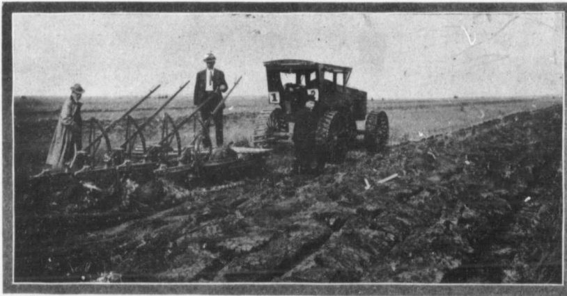
The Canadian Heer 20-25 Kerosene Tractor pulling a Four Bottom Cookshutt Engine Gang.
