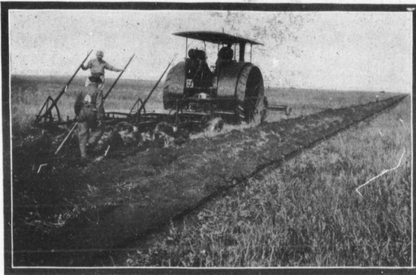
The Aultman and Taylor Kerosene Tractor pulling seven John Deere Bottoms, (Silver Medal winner Class E.)
