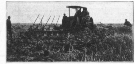
The Rumely 10 bottom engine gang in the Winnipeg Plow Competition going through a bunch of wolf willow. Note that there is no clogging, and that the willows are being thoroughly buried.
