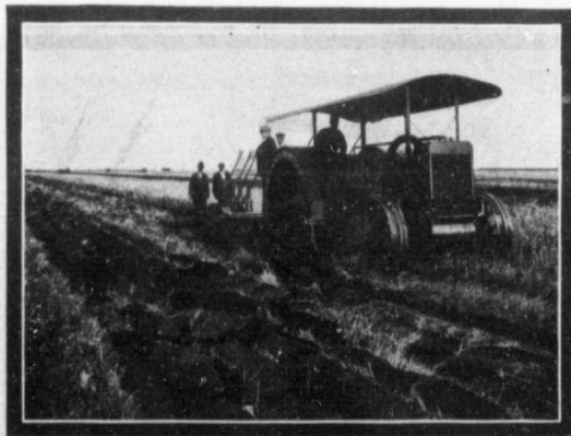
The Gould Shapley and Muir "Ideal" Tractor pulling a four bottom Cockshutt Engine Gang. (Silver medal winner Class B.)
