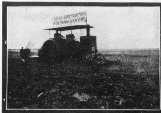
The Aultman & Taylor 30-60 Gasoline Tractor pulling a Nine Bottom John Deere Engine Gang. (Gold medal winner Class C.)
