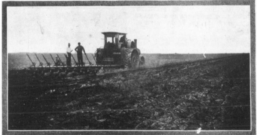
The Case 110 h.p. Steam Tractor pulling a Case-Sattley 12 bottom Engine Gang (Gold Medal winner Class B)
