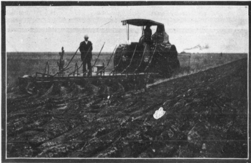
The Rumely 30-60 Oil-Pull Tractor pulling an Eight Bottom Engine Gang. (Gold medal winner Class E)
