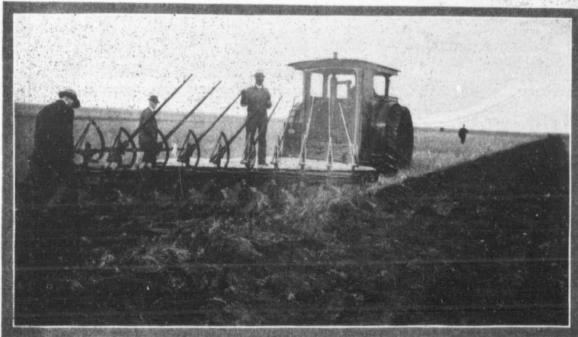
The I. H. C. 45 H.P. Gasoline Tractor pulling a nine bottom P. &amp; O. Engine Gang.
