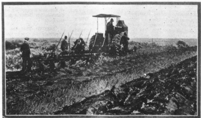
The Rumely 15-30 Oil-Pull handling a nice patch of Wolf Willow in the Plow Contest. A Rumely Six Bottom Engine Gang is being pulled. This plow won Silver Medal in Class B.
