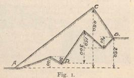
A foot of rise and fall means one foot of rise and one foot of fall, going in one direction only. Thus in Fig. 1, the total rise and fall between "A" and "B" by either route equals 710 feet.
