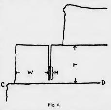
and the length of line of least resistance. The diameter of the hole, as shown before, depends upon its length. The reduction in the length of the charge, M, calculated in the ordinary way, is regulated as follows, T being the thickness of the stratum, M the calculated length of charge,  $M_1$
