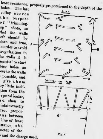
V-SHAPED CENTER CUT. In Fig. 8 is shown the V-cut, which offers two advant-
