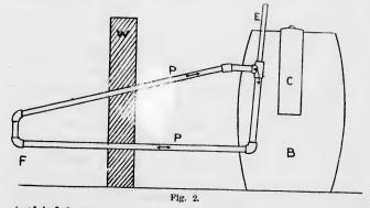
A third form which is recommended by Mr. Brainerd of the Hamilton Powder Co. for thawing large quantities of dynamite at a time consists of a barrel B (Fig 2)
