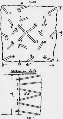
9 and 11. All the enlarging shots are breaking to two free faces, being nearly the equivalent of bench blasting, and they all have relatively short lines of
