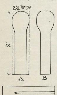
Illustration No. 2—Block of wood and nail to make the groove. A shows the label marked out on a strip of zinc. B shows the label finished with groove in the shank.
