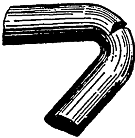
FIG. 9.—SHARP BEND IN A WIRE.
