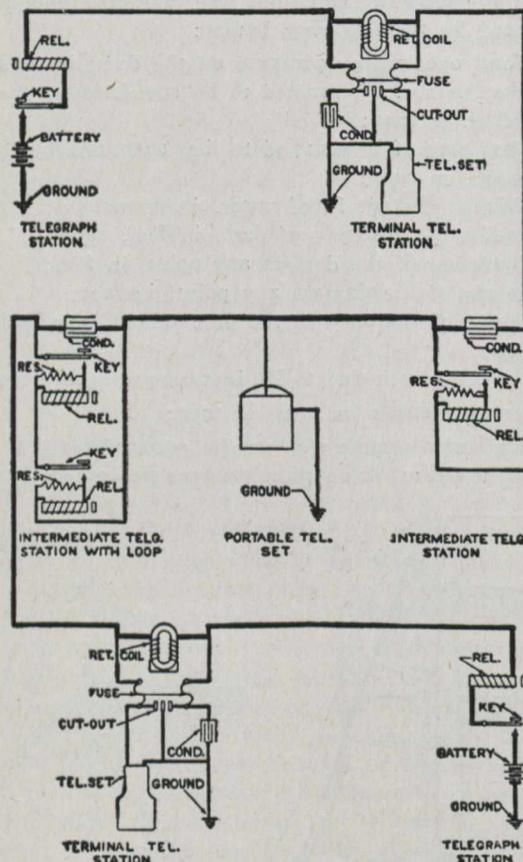
**SIMPLIFIED ARRANGEMENT OF LINE RAILWAY COMPOSITE SYSTEM.**
