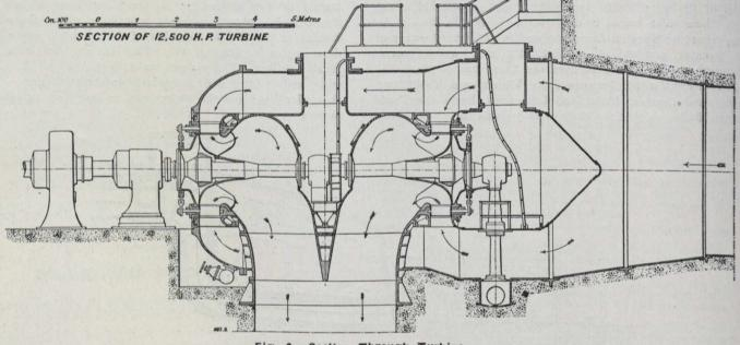
Fig. 2.-Section Through Turbine.
