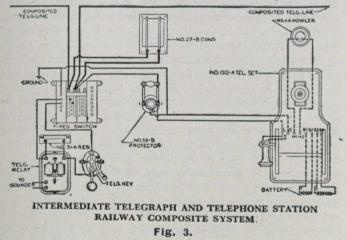
is a whistle or shriek, whose tone can be adjusted to any pitch by the adjustment of the diaphragm. In each composite set an interrupter on the induction coil is used to furnish a high frequency signalling current from a small battery of dry cells. A push button on the side of the 1312-A wall set allows the person calling to ring any code with the greatest ease.
