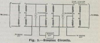
In its operation, the telegraph currents traverse the two wires and two winding of each coil as parallel branches of the one circuit. The telephone currents are repeated through the different repeating coils just as the currents of a lighting transformer are. Upon the efficiency of this repeating coil for voice currents depends the transmission of the conversation.
