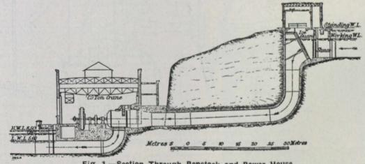
Fig. 1.-Section Through Penstock and Power House.
