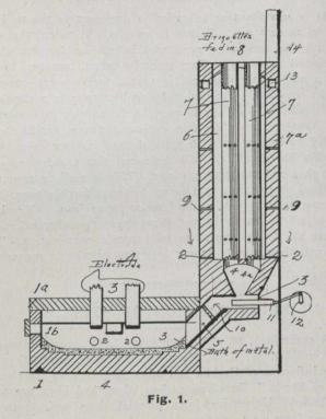
electric furnace and from the briquettes themselves are burned round these pipes and serve to heat them. The ore in the presence of carbon becomes reduced to metal, and finally is charged by the mechanism shown into the electric furnace. Fig. 2 is a photograph of an electric furnace with a tower for the reduction of the ore.
