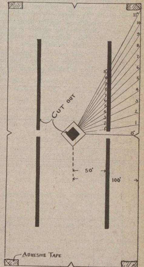
PAPER PROTRACTOR FOR PLOTTING CROSS SECTIONS FROM CLINOMETER READINGS; VERTICAL SCALE TEN TIMES HORIZONTAL SCALE
