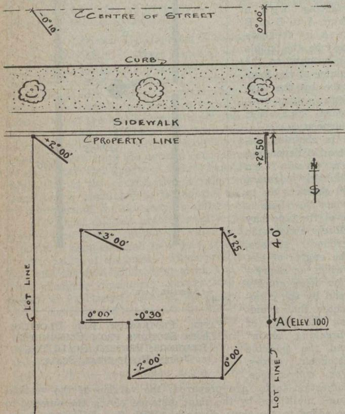
TYPICAL FIELD NOTES FOR THE DETERMINATION OF GROUND ELEVATIONS BY CLINOMETER READINGS
