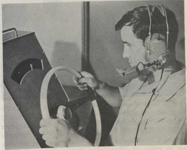
*Subject tracks moving light on the stressalyzer as engineers and psychologists in the Control Systems Laboratory record his reaction and movement times.*
