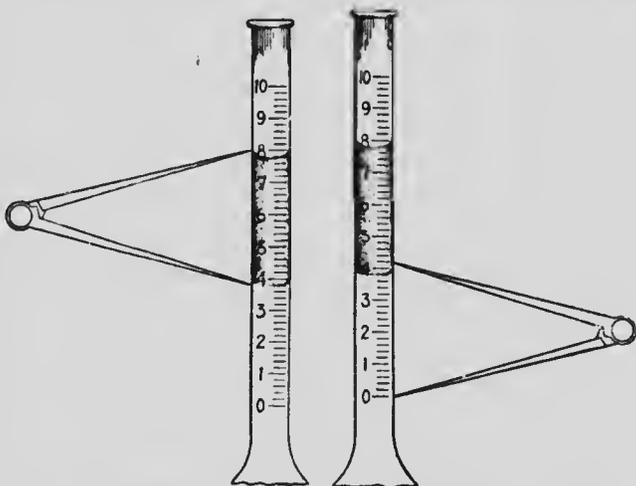
THE DIVIDERS IN THE FIRST POSITION FOR READING THE TEST
