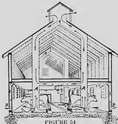
Showing a pair of U-shaped outtakes adapted to stables of 60 to 80 cows. A A A A are the outtakes; B B B B are the intakes; C, ceiling register in a cross-arm joining the two sides of the outtake, to be opened when needed for cooling the stable and re-inforcing the draft. (From "Ventilation for Dwellings, Rural Schools and Stables", by F. H. King.)
