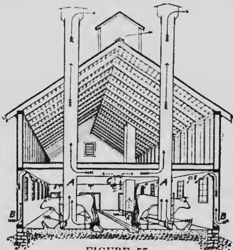
Showing single straight-away outtakes which avoid all angles and render possible the strongest draft. A A are the two outtakes; B B are the intakes; C, a ceiling register in the cross-arm joining the two sides of the outtake. (From "Ventilation for Dwellings, Rural Schools and Stables", by F. H. King.)
